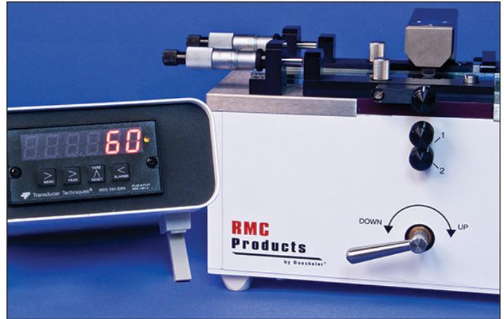
*The GKM-2 glass knife maker by RMC Products includes a digital readout that displays the load applied to glass as the breaking arm is moved.*
