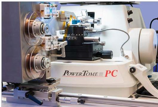
The ATUMtome automated tape collecting ultramicrotome manufactured under license by RMC Products by Boeckeler Instruments Inc.
